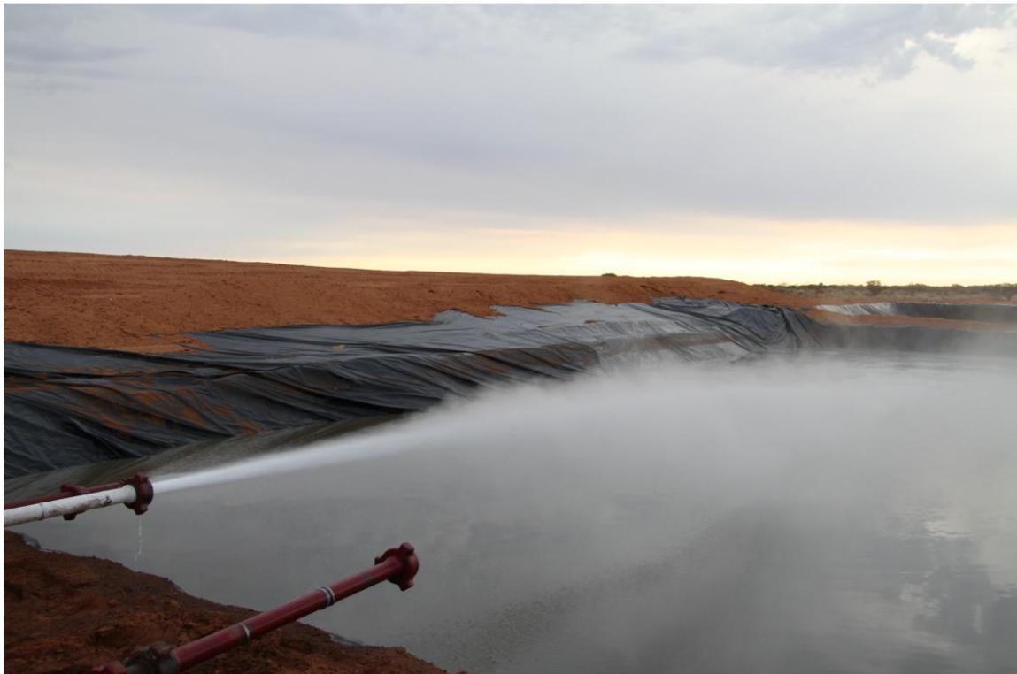
Hot fluids (water and steam) from the Paralana 2 well flowing into a containment pond
