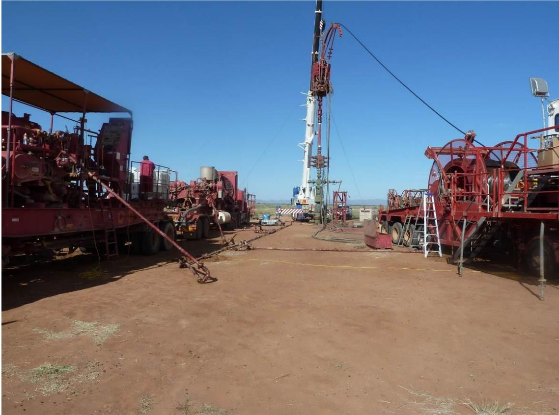
**Figure 1** Recent operations at Paralana well site. Coiled tubing unit in operation (right) replacing brine fluid with water. Injection Pumps (left) set up in readiness to perform injectivity test.
