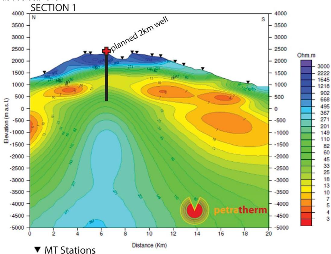
**Figure 2:** Section 1: North-South resistivity cross-section, showing projection of a planned 2km slim-hole well
