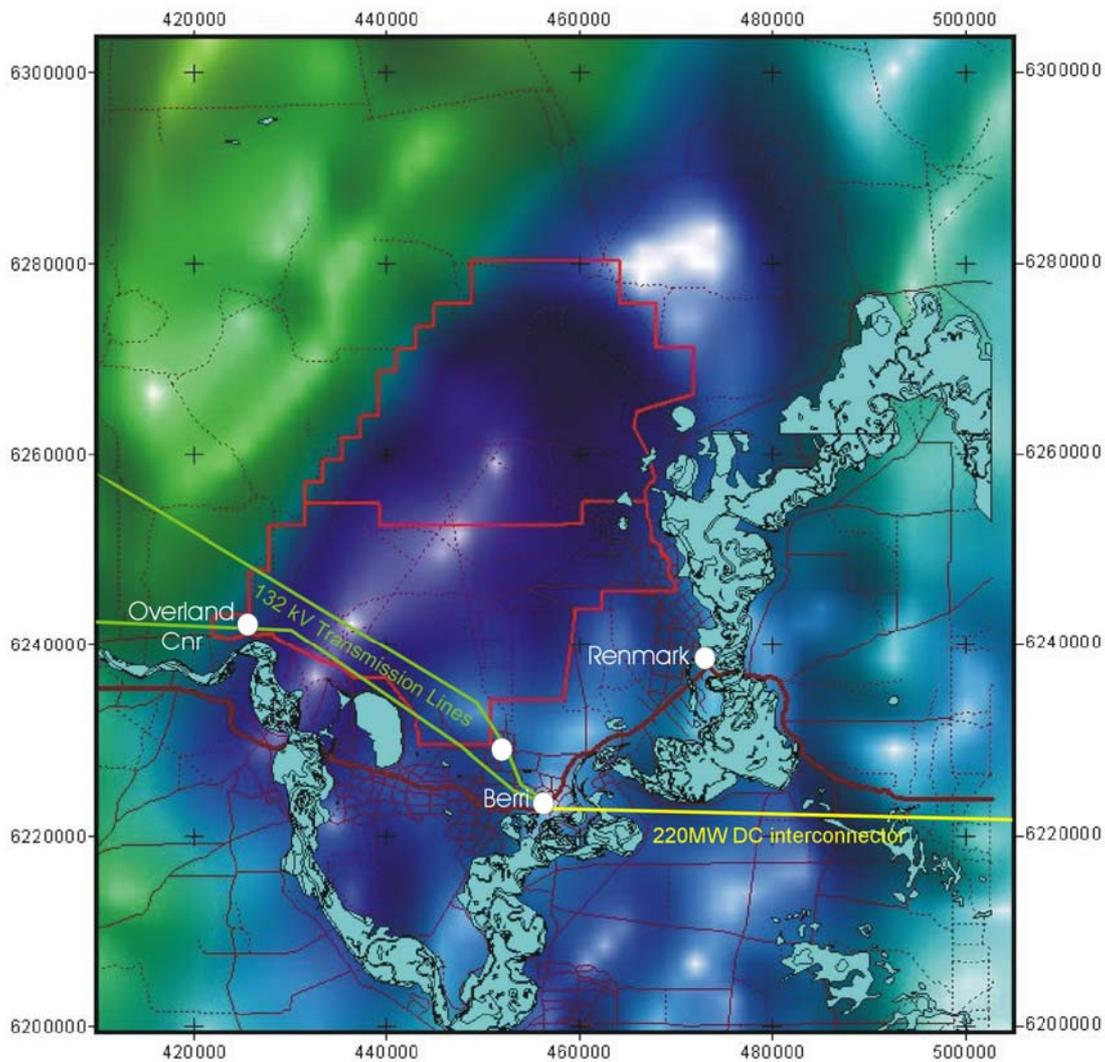
**Map 2** A gravity image of the Renmark area indicating the location of the new GELs and their relationship to transmission infrastructure and townships. The dark blue shadings on the gravity image represent the deepest, and thus the most prospective portions of the Renmark Trough. The boundaries of the GELs are outlined in red and clearly bracket the deepest parts of the sub-basin.
