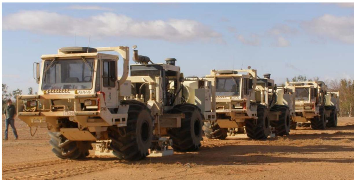
**Figure 1. Vibroseis trucks in operation at Paralana**
